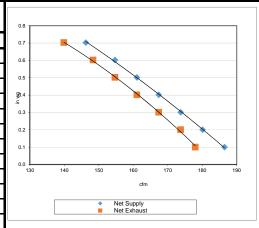
NOTE: FAN CURVE PERFORMED ON HIGH SPEED
