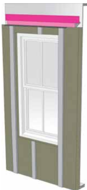
Step 17: Sheathing tape applied over adhesive membrane strip to secure top edge.
