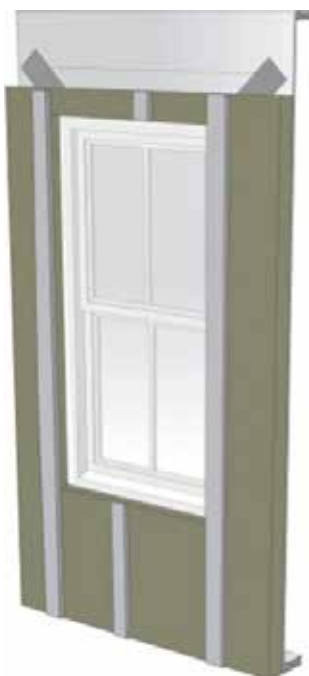
Step 14: Install furring over ROXUL COMFORTBOARD 80 insulation.
