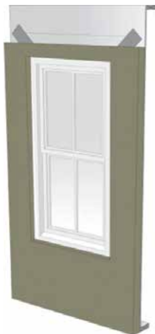
Step 13: Install ROXUL COMFORTBOARD 80 insulation.
