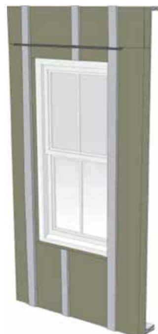
Step 18: Install next course of ROXUL COMFORTBOARD 80 and furring. Drainage gap created by furring. Do not fasten furring through head cap flashing.
