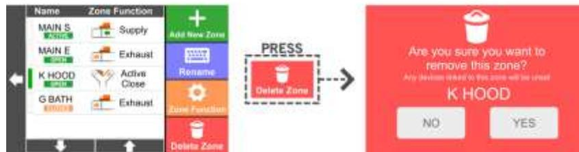
Note: when deleting a zone, any auxiliary inputs or wireless devices linked to this zone will revert to controlling the CERV as a whole (i.e. triggering a ventilation switch would ventilate the whole home instead of the previous zone). Any auxiliary outputs configured as Zone Dampers linked to this zone will be unset.
