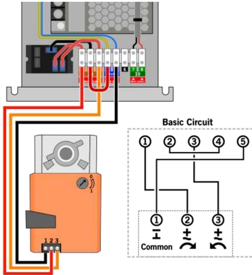
The terminal block for the X0 Auxiliary Output is located in the bottom section of the CERV2 (**see appendix at end of document for access instructions**). Because the X0 is a standard dry contact with Normally Open (1), Common (2), and Normally Closed (3) terminals, it must be used in conjunction with the 24VAC output terminals (4, 5) as seen above.
