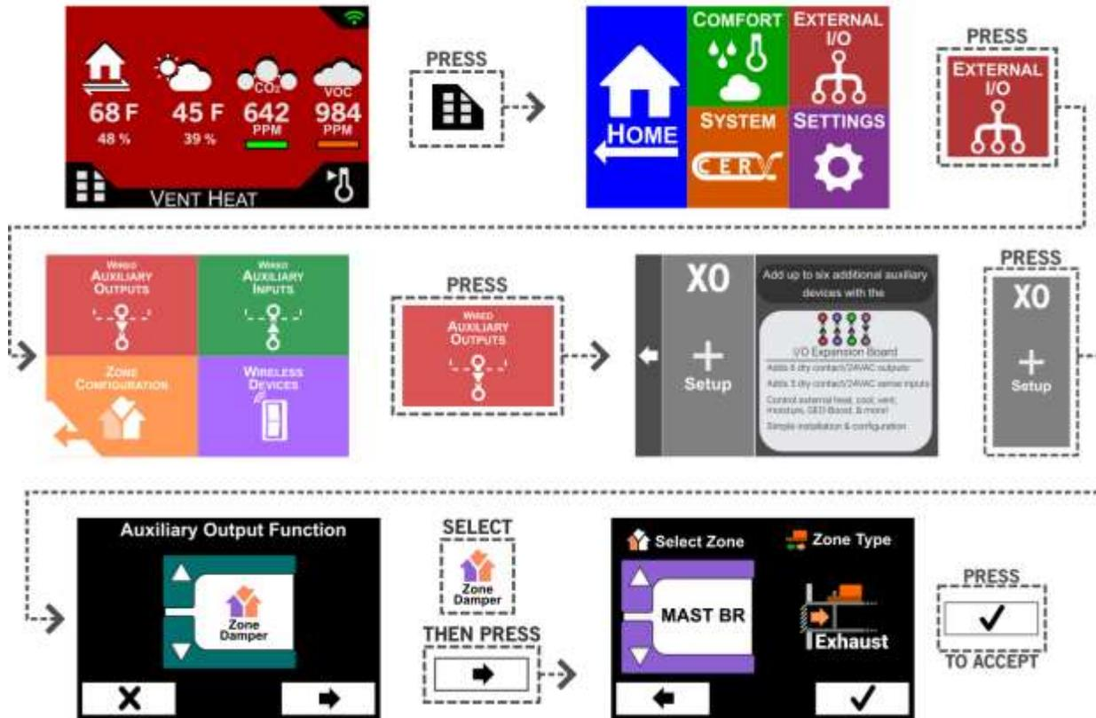
After an auxiliary output has been set to actuate a damper motor, you may configure inputs to trigger one of your configured zones. The steps below walk through setup of wired auxiliary inputs (I0, or I1-I3 on the IO Expansion Board), as well as wireless options such as the wireless ventilation switch or active circuit transmitter. Note: If no zone selection is made, the input will trigger the CERV as a whole to ventilate. Additionally, multiple zones may be linked to the same input if desired
