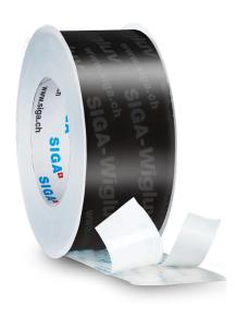
Semi-permeable special PO film • UV exposure: 12 months • 1.7 US perms • The bond must not be under standing water • Suitable for open facades with up to 2" joint width and a max. proportion of 40%.
