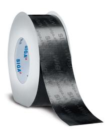
Semi-permeable special PO film • UV exposure: 12 months • 1.7 US perms • The bond must not be under standing water • Suitable for open facades with up to 2" joint width and a max. proportion of 40%.
