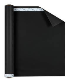
2-ply membrane: acrylate coating on robust polyester fleece • Thickness 20 mils • Fire behavior: Class A (ASTM E84) • 107 US perms (ASTM E96 Method A) • Suitable for open facades with up to 2" joint width and a max. proportion of 40%.
