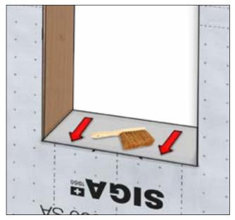
Fix sloped sill material to sill as per project specification. Clean area from dust and debris.
