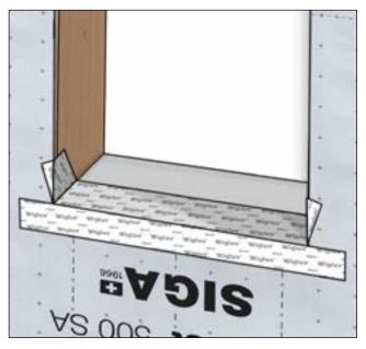
Cut Wigluv 4" wider than the sill so it will extend 2" past each end of the rough opening. Flash sill as usual while cutting the tape lengthwise toward the corners.
