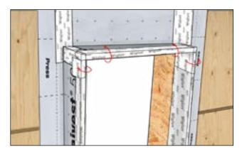
Flap ends around extension buck and apply even pressure. Don't overstretch tape.
