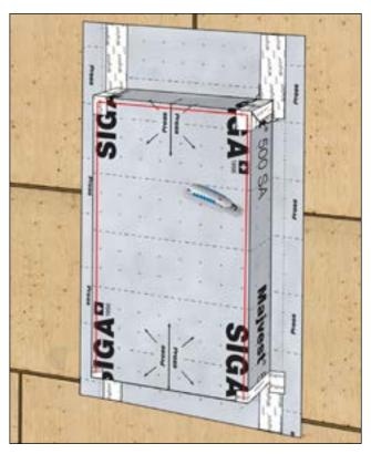
Cut out membrane while using the inner edge of jambs and head as a guide.
