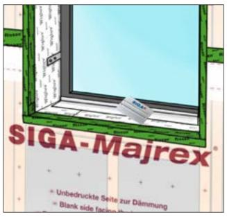
Remove backing paper and apply firm pressure using a roller or squeegee.
