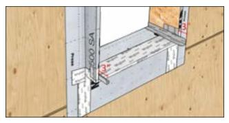
Create two gussets with Wigluv 100 by cutting a piece of tape that's the full depth of the rough opening plus 3".
