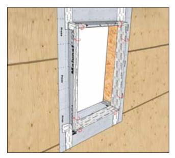
Flap ends around extension buck and apply even pressure. Don't overstretch tape.
