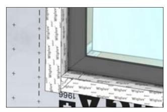
**OPTIONAL** Dependent on window type the sill can either be taped or left open for drainage. Check with your window manufacturer before taping.
