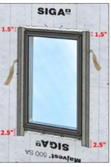
Apply Fentrim 430 grey along jambs while overlapping 1.5" on top and 2.5" on the bottom while removing one backing strip.
