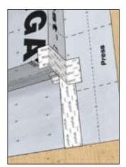
Apply tape around horizontal portion overlapping about 2" around each corner.
