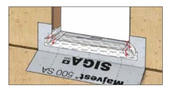
Stretch the Wigluv tape around the corner toward the exterior — wrinkles are normal!
