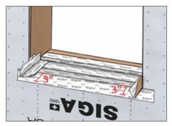
Create two gussets with Wigluv 100 by cutting a piece of tape that's the full depth of the backdam plus 3". Cut one end of the tape at a 45 degree angle to create a "dog ear".
