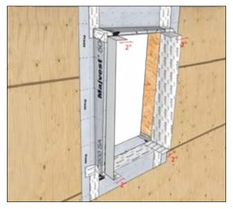
Cut Wigluv 4" wider than the jamb so it will extend 2" past each end of the rough opening.
