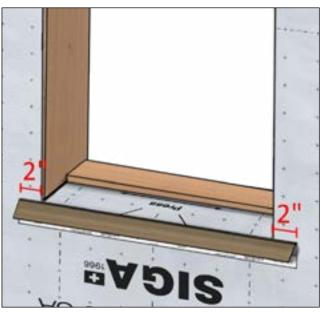
Cut Wigluv 4" wider than the sill so it will extend 2" past each end of the rough opening. Crease the tape using the split backing and remove one backing strip.
