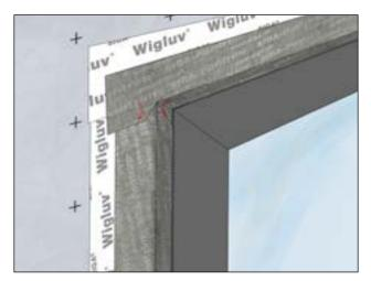
Fold both ends up and apply firm pressure. Repeat on both sides.
