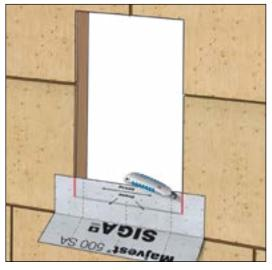
Cut along jambs into the corner while using the sheathing as a cutting guide.
