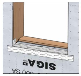
Flash sill as usual while cutting the tape lengthwise toward the corners.
