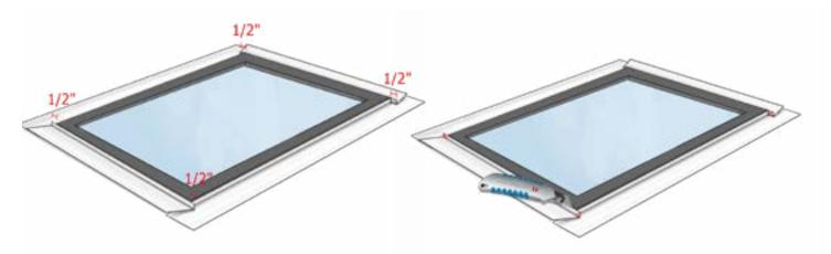
Apply Fentrim IS 20 on top and bottom of frame while making sure all tapes line up — overlap  $\frac{1}{2}$ " on each side.
