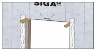
Work both gussets in top corners while removing one backing strip.
