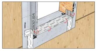
Flap ends around extension buck and apply even pressure. Don't overstretch tape.
