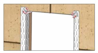
Stretch the Wigluv tape around the corner toward the exterior — wrinkles are normal!
