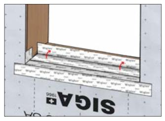
Remove backing paper and fold up while working the tape tightly in the corner using a squeegee.
