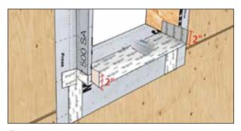
Cut Wigluv 4" wider than the sill so it will extend 2" past each end of the rough opening.
