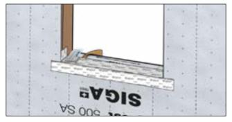
Remove second backing strip and apply tape on sill. Firmly press the tape on with a roller or squeegee.
