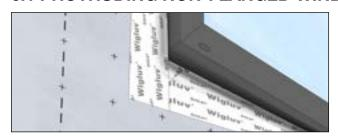
**OPTIONAL** Dependent on window type the sill can either be taped or left open for drainage. Check with your window manufacturer before taping.
