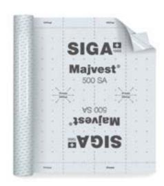
microporous PP sheet with full-coverage adhesive on reverse Thickness: 28 mils • Installed Weight per unit area: 0.84 oz/sq ft UV stable: 6 months (IECC zones 3-8) • Fire behavior: Class A (ASTM E-84) • 16 US perms (ASTM E96 Method A)
