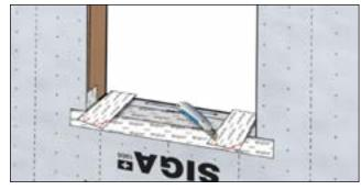
Cut one end of the tape at a 45 degree angle to create a "dog ear."
