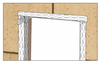
Remove second backing strip and apply tape on head while firmly pressing on with a roller or squeegee.
