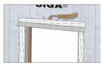
Crease along split backing and remove one backing strip.
