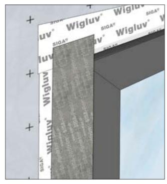
Cut Fentrim 430 grey about 4" wider than the width of the prepared rough opening so both ends are overlapping the tape on the jamb.
