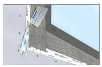
Remove second backing paper and press on firmly using a roller or squeegee.
