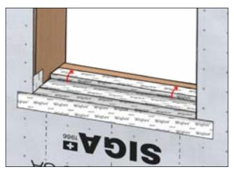
Flap over rest of tape while applying even pressure.
