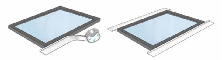
Bond the narrow side of Fentrim IS 20 on the length of the window with an extension corresponding to the width of the Fentrim IS 20 past each end. Press on firmly.
