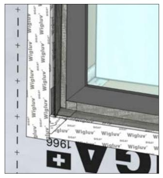
Cut Fentrim 230 grey the same length as the vertical portion of the rough opening. Apply pre-folded section of the tape along vertical portion of the window frame.
