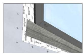
Cut Fentrim 430 grey about 2" wider than the width of the prepared rough opening. Remove one backing paper and apply the tape along underside of the window while applying firm pressure.
