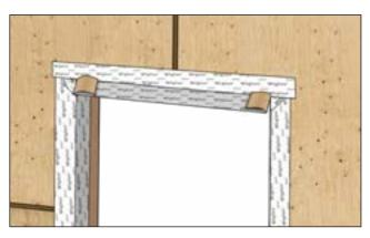
Flap ends up and fold tape into the head.
