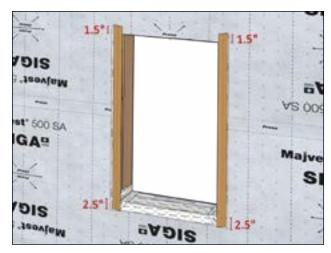
Cut Wigluv +4" longer than jambs to extend 1.5" on top and about 2.5" on the bottom.
