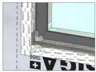
Apply 3D corner boot in bottom corner while applying firm pressure — repeat on both sides.
