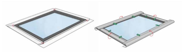
Bond flaps of the narrow tape to the window frame.
