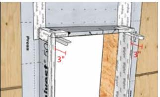
Create two gussets with Wigluv 100 by cutting a piece of tape that's the full depth of the rough opening plus 3".
