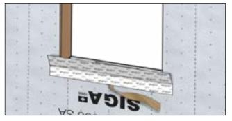
Crease the tape using the split backing and remove one backing strip. Center and apply to exterior face.
