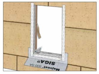
Remove second backing strip and apply tape on jambs while firmly pressing on with a roller or squeegee.
