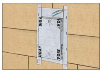
Cut the protruding Majvest 500 SA flaps so that the WRB lines up horizontally.
