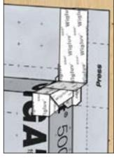
Tape membrane with Wigluv 100 and overlap corner piece.
