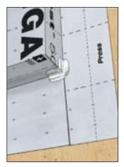
Use 4" long tape strip and apply into corner while using the stretch of Wigluv. corner piece from below.
