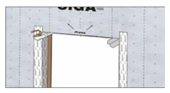
Press on firmly using a roller or squeegee.
