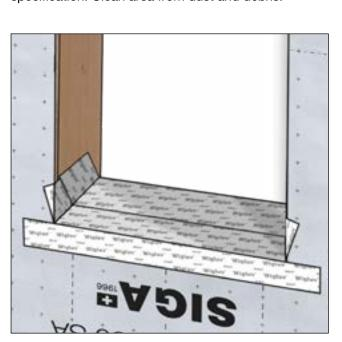
Add another tape layer if needed to extend past inner surface of installed window.
