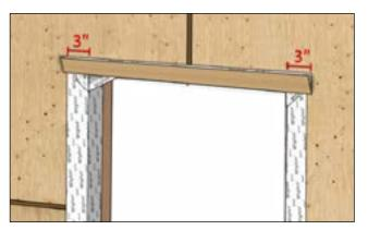
Cut Wigluv +6" wider than head to extend 3" past each end.
