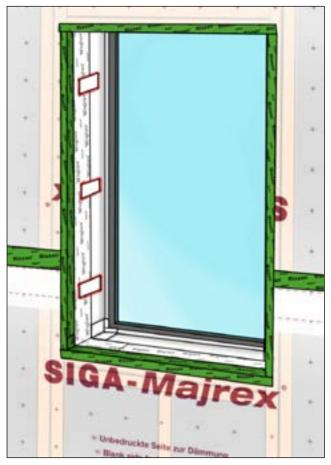
Tape around the interior face of the window, and seal the mounting brackets or any other possible sources of leakage.
