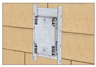
Fold front pieces in on top and press on firmly. **Do not** press on bottom flap to the substrate as the field membrane will later be integrated below.
