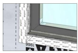
Cut Fentrim 230 grey the same width as the prepared rough opening. Apply narrow side of the tape along the window frame while applying firm pressure.
