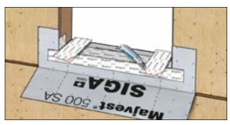
Cut one end of the tape at a 45 degree angle to create a "dog ear."
