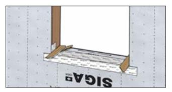
Work gusset into corner while removing one backing strip.
