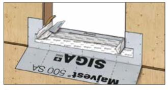
Firmly press the tape onto the rough opening using a roller or squeegee.
