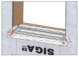
Use stretch of Wigluv tape and work around corner. Press on firmly using a roller or squeegee — wrinkles are normal!
