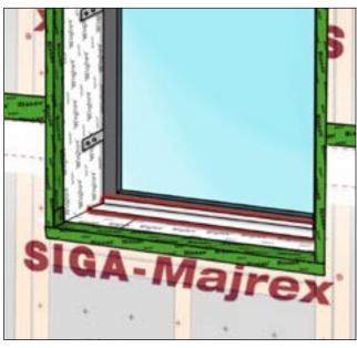
Apply Fentrim IS 20 directly on window frame with the pre folded section.
