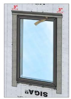
Cut Fentrim 430 grey +6" wider than rough opening to overlap 3" on each side. Apply tape along top of the window while removing one backing strip.
