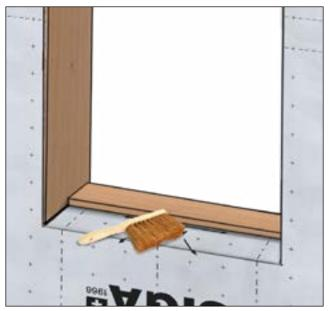
Fix backdam material to sill as per project specification. Clean area from dust and debris.
