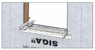
Firmly press the tape onto the rough opening using a roller or squeegee.
