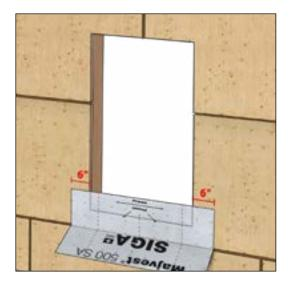
Install 18" Majvest 500 SA detail roll above the sill plate with a distance same as the sill depth. Cut membrane +12" wider than sill to extend 6" past each end.
