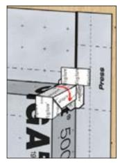
Fold remaining tape section onto the exterior jamb of the extension buck. Apply pressure.
