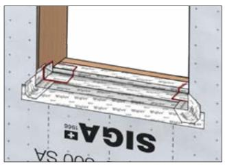
Install 3D corner boot shown on page 32. Press on firmly using a roller or squeegee.
