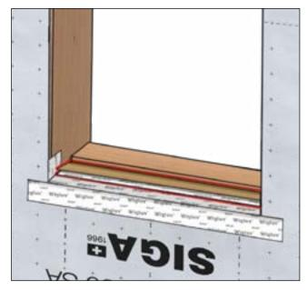
Add tape the same width as the sill and overlap 1" onto the pre-flashed part.
