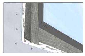
Cut Fentrim 430 grey about 2" wider than the vertical portion of the rough opening. Remove one backing paper and apply the tape along the vertical portion of the window while applying firm pressure.
