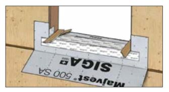
Work gusset into corner while removing one backing strip.
